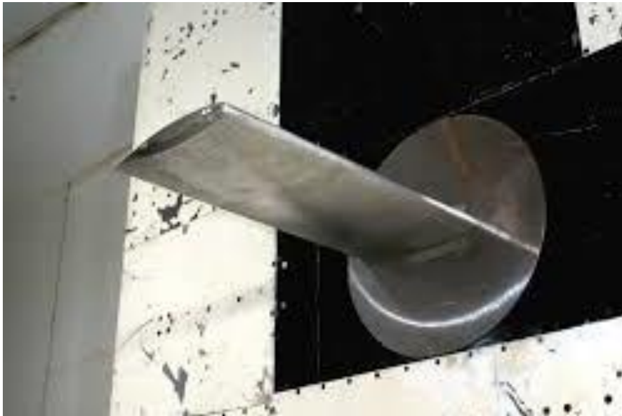
BSCW mounted in TDT at NASA LaRC
