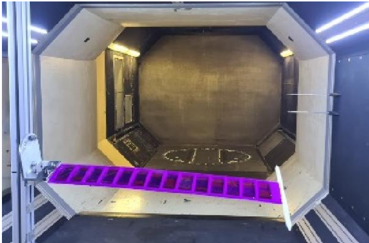
The Sapienza Pazy wing in the SOTON 7x5 wind tunnel [REF]
