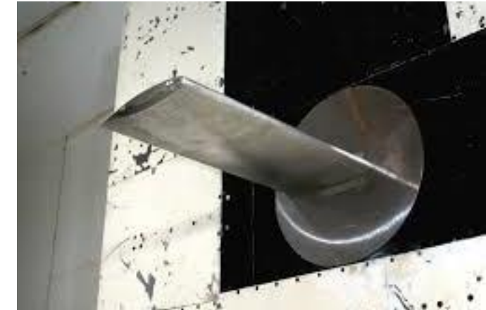
BSCW mounted in TDT at NASA LaRC
