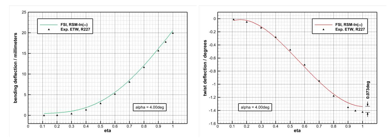
Deformation Data obtained from the Trans National Access (TNA) Test Campaign (2012), European Transonic Wind Tunnel (ETW), Cologne, Germany.
