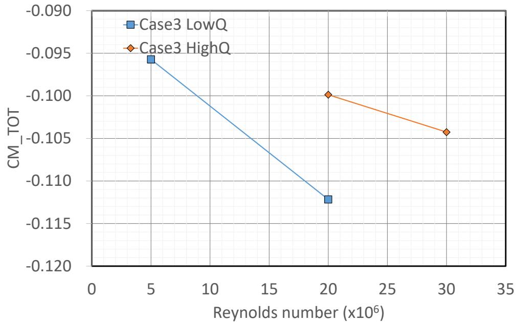
Some jumps are found at  $Re=20M$  by the difference of  $Q$  especially for  $CD_{PR}$  and  $CM$
