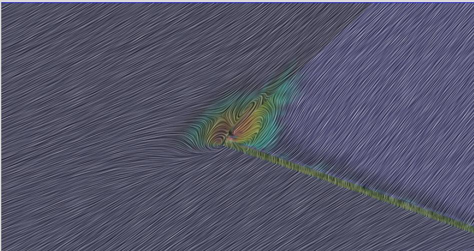
SOB separation is present although medium/fine meshes are needed to assess its trend with mesh refinement
