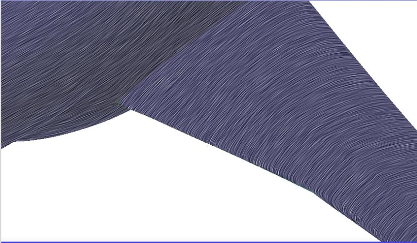
Rest of the plane is clean with the only expected separation in the junction region
