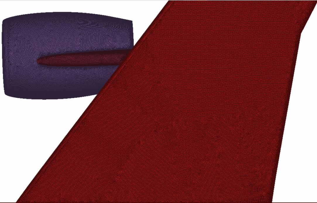
Based on initial CFD runs the path of the tip vortex was meshed with a pure hexa mesh
