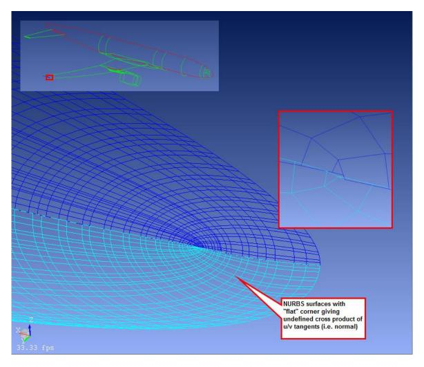
The localised twisting of the NURBS surface at the flat corner has been smoothed out in all the deformed configurations.
