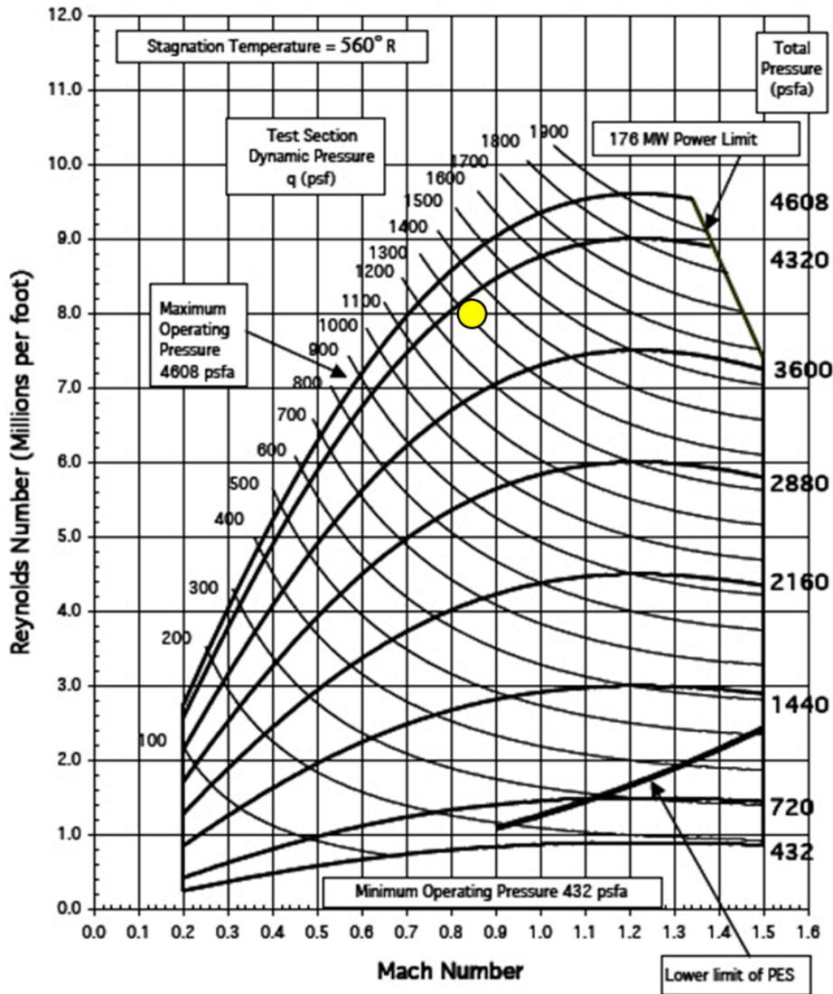
Figure 20: Ames 11-ft WT Operating Chart with CRM  $Rn_c=5$  million Test Condition.
