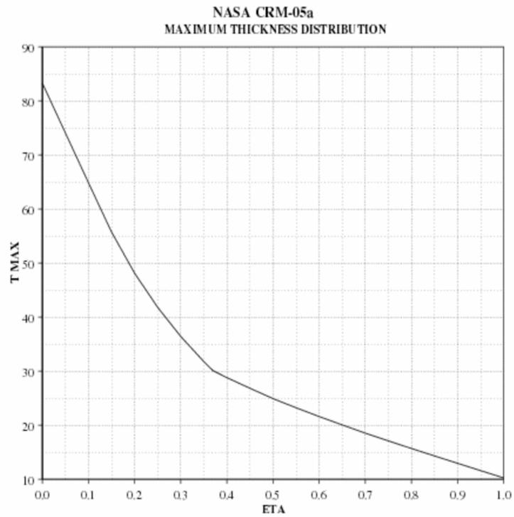
Figure 4: Dimensional Thickness Distribution of the CRM Wing.
