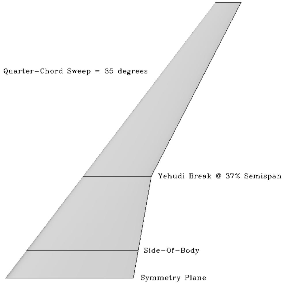
Figure 1: Full-Scale Planform of the CRM Wing.
