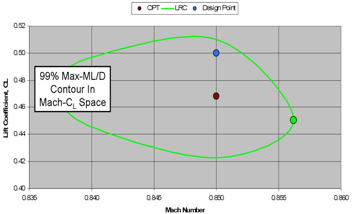
Figure 16: Contour of 99% Max-ML/D for the CRM Wing/Body.
