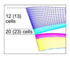
Trailing edge closed with Bézier-splines (AIAA-95-0089), camberline retained
